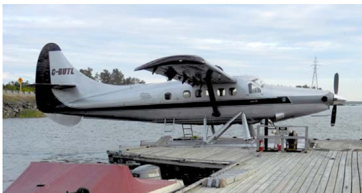
C-GUTL was built as a piston Otter in 1960 and was flown by the RCAF until 1981. Following a crash in 1998 when it was owned by Fort Frances Sportsmen Airways it was rebuilt as a Turbo Otter and now flies with Northern Wilderness Outfitters of Fort Frances.
